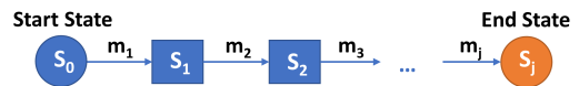
Figure 5: Finite state machine (FSM) representing DOM tree status transitions via mutations m_1, m_2, \dots, m_j .
